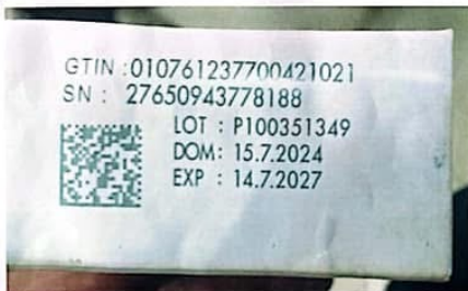
Picture 2: Folding box lid containing the variable data. The variable data imprint is the most obvious irregularity for this unit. The GTIN is longer, than expected. The data matrix code contains the following information: "010761237700421021276509437781881724070810P100378987" and is not consistent with the lot # and expiry date written in plain text next to it. The serial number belongs to the genuine CSL Behring Rhophylac® lot # P100378987, that has been delivered to Egypt and Jordan.
